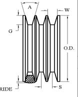
The length shall be measured by placing the belts on two sheaves of equal diameters that have been grooved in accordance with standard specifications and rotated at least three complete turns with the specified tension so that each strand receives half the total tension. The length will be that length obtained by adding the Reference Circumference of one sheave at dimension 'W' to twice the center distance (dimension 'Y').
