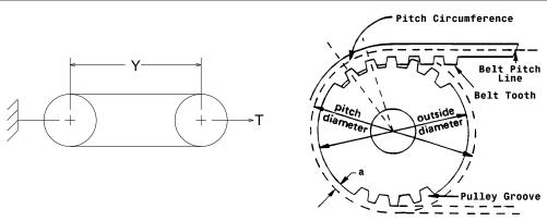
The length shall be measured by placing the belts on two pulleys of equal diameters that have been grooved in accordance with standard specifications and rotated at least three complete turns with the specified tension so that each strand receives half the total tension. The length will be that length obtained by adding the Pitch Circumference of one pulley to twice the center distance (dimension 'Y').
