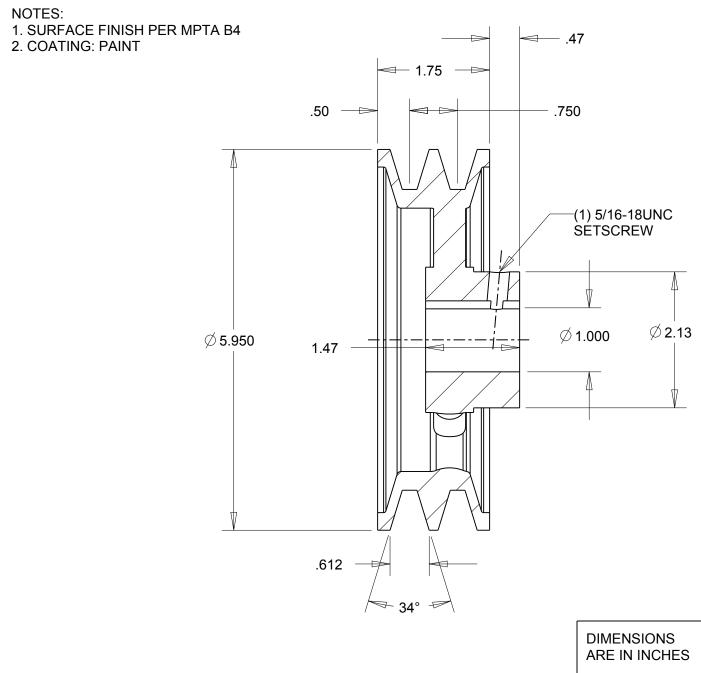
This drawing is a stock power transmission component. Details shown which do not affect drive function may be changed without any notification.
