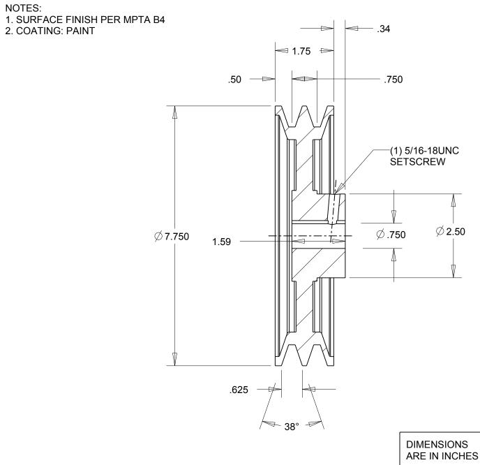
Denver, Colorado 2BK80.3/4 **IRON** Gates Part No: Material: Finish: **PAINT** 78057321 This drawing is a stock power transmission component. Details shown which do not affect Gates Product No: drive function may be changed without any notification.
