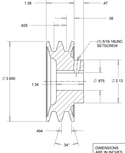
**Gates Corporation** ARE IN INCHES Denver, Colorado **IRON** Gates Part No: 2AK41.7/8 Material: Finish: **PAINT** 78070173 This drawing is a stock power transmission component. Details shown which do not affect Gates Product No: drive function may be changed without any notification.
