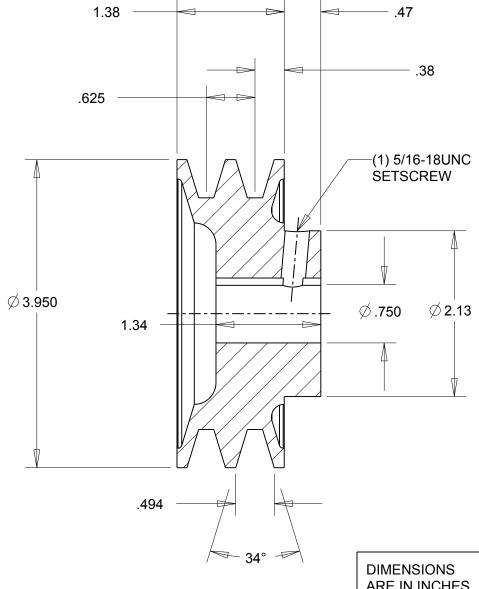
**Gates Corporation** ARE IN INCHES Denver, Colorado **IRON** Gates Part No: 2AK41.3/4 Material: Finish: **PAINT** 78070172 This drawing is a stock power transmission component. Details shown which do not affect Gates Product No: drive function may be changed without any notification.
