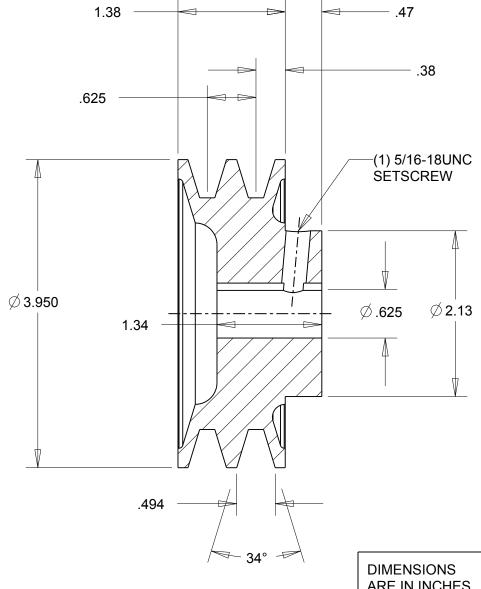
**Gates Corporation** ARE IN INCHES Denver, Colorado **IRON** Gates Part No: 2AK41.5/8 Material: Finish: **PAINT** 78070171 This drawing is a stock power transmission component. Details shown which do not affect Gates Product No: drive function may be changed without any notification.
