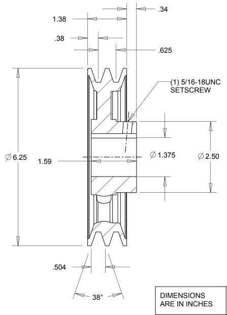
**Gates Corporation** Denver, Colorado **IRON** Gates Part No: Material: 2AK64 1.3/8 Finish: **PAINT** 78050256 This drawing is a stock power transmission component. Details shown which do not affect Gates Product No: drive function may be changed without any notification.
