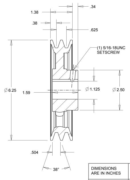
Material: Finish: This drawing is a stock power transmission component. Details shown which do not affect drive function may be changed without any notification.
