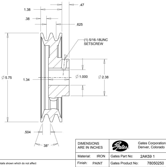
This drawing is a stock power transmission component. Details shown which do not affect drive function may be changed without any notification.
