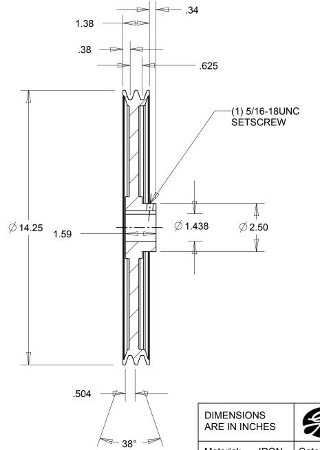
This drawing is a stock power transmission component. Details shown which do not affect drive function may be changed without any notification.
