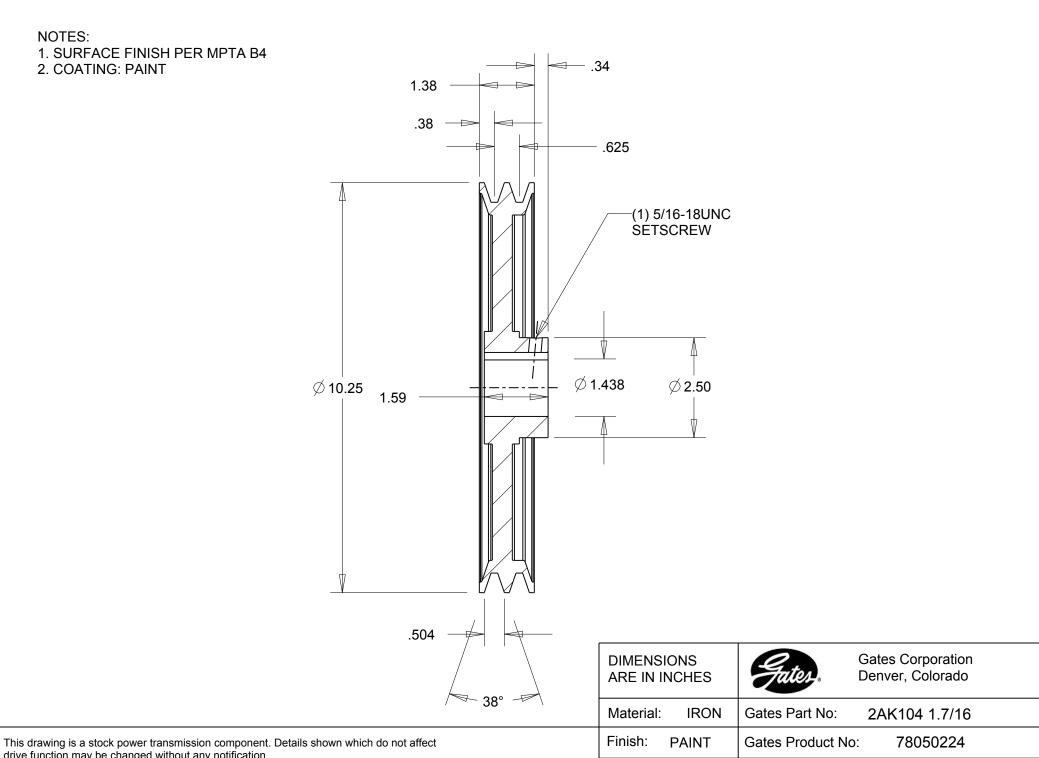
this drawing is a stock power transmission component. Details shown which do not affect drive function may be changed without any notification.
