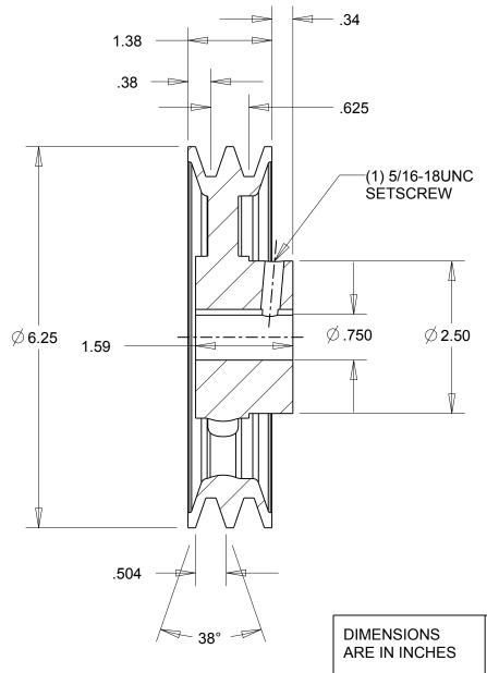
**Gates Corporation** Denver, Colorado **IRON** Gates Part No: Material: 2AK64.3/4 Finish: **PAINT** 78050200 This drawing is a stock power transmission component. Details shown which do not affect Gates Product No: drive function may be changed without any notification.
