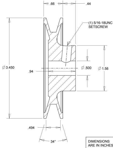
This drawing is a stock power transmission component. Details shown which do not affect drive function may be changed without any notification.
