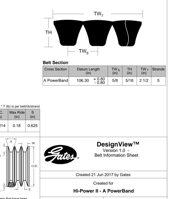
The length shall be measured by placing the belts on two sheaves of equal diameters that have been grooved in accordance with standard specifications and rotated at least three complete turns with the specified tension so that each strand receives half the total tension. The length will be that length obtained by adding the Reference Circumference of one sheave at dimension 'W' to twice the center distance (dimension 'Y').
