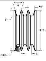
The length shall be measured by placing the belts on two sheaves of equal diameters that have been grooved in accordance with standard specifications and rotated at least three complete turns with the specified tension so that each strand receives half the total tension. The length will be that length obtained by adding the Reference Circumference of one sheave at dimension 'W' to twice the center distance (dimension 'Y').
