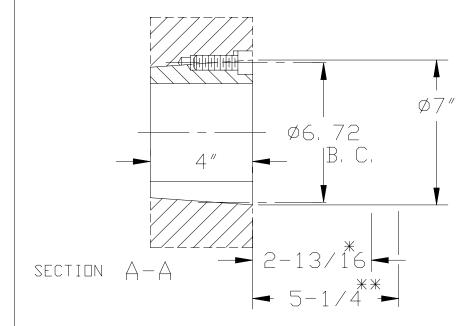
\* SPACE REQD TO TIGHTEN BUSHING ALSO SPACE REQD TO LOOSEN SCREWS TO PERMIT REMOVAL OF HUB BY PULLER.
