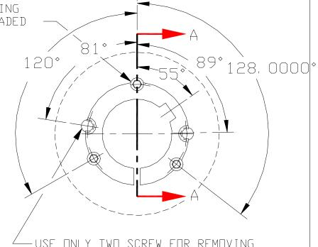
BUSHING HALF OF HOLE IS THREADED-HUB HALF OF HOLE IS NOT THREADED BURE: BUSHING KW:
