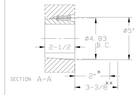
\* SPACE REQD TO TIGHTEN BUSHING ALSO SPACE REQD TO LOOSEN SCREWS TO PERMIT REMOVAL OF HUB BY PULLER.
