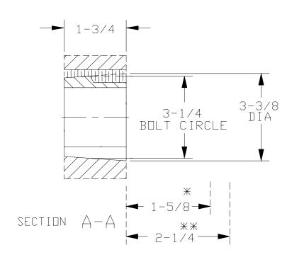
\* SPACE REQD TO TIGHTEN BUSHING ALSO SPACE REQD TO LOOSEN SCREWS TO PERMIT REMOVAL OF HUB BY PULLER.
