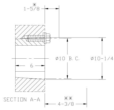
\* SPACE REQD TO TIGHTEN BUSHING ALSO SPACE REQD TO LOOSEN SCREWS TO PERMIT REMOVAL OF HUB BY PULLER
