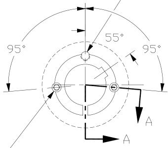
(2) 5/8-11 NC X 1-1/4 LG SET SCREWS FURN W/ BUSH TO TIGHTEN ON SHAFT (HUB HALF OF HOLE IS THREADED & BUSH HALF OF HOLE IS NOT THREADED)
