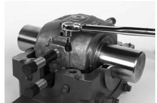
**NOTE:** If liner cap on non-expansion bearing will not drop into place, remove cap and reposition thrust plates tightly against thrust collar. Reinstall liner cap.
