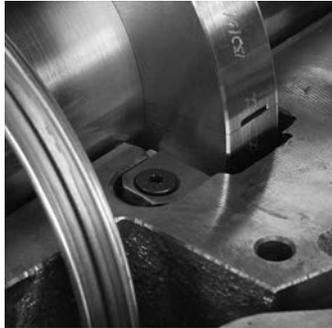
Place the other thrust plate half (half with two milled slots in steel back) against thrust collar, making sure babbitt faces thrust collar.
