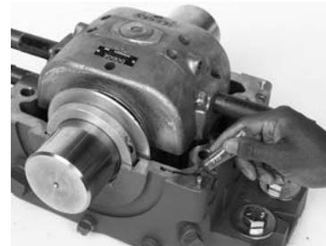
The plunger screw must remain loose until the housing bolts have been tightened.
