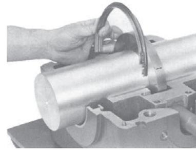
Install oil ring screws to insure they are secure. Repeat for second ring.
