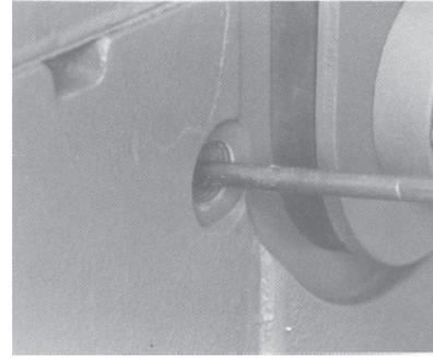
Check construction drawings to determine if coolant (water or air) is to be supplied to the bearings. Do not connect coolant pipes and bearing unless construction drawings and/or equipment instructions call for this. If no connection is required, pipes can be left open.
