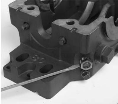
Apply oil to the spherical seats of the housing base.
