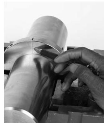
Tighten set screws to value specified in Table 1. **Install and tighten jam screws 1/10 of torque specified for set screws.**
