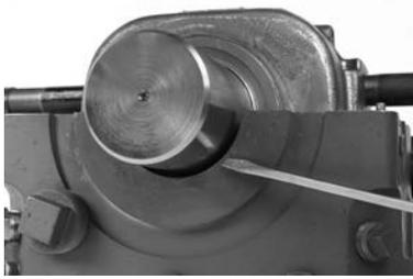
Tighten the four pedestal bolts to torque value given in Table 3. Shaft should rotate freely.
