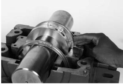
Install retainer washer in groove in liner base. Rotate plate until stopped by retainer washer.
