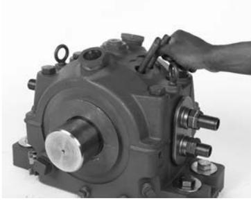
Install grommet, grommet plate and collar over each inlet pipe. Press down on collar and tighten collar set screw.
