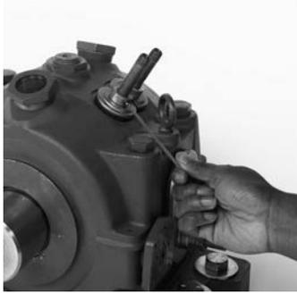
**NOTE: ALL plumbing (oil and water) should be cleaned and flushed before being connected to the pillow block. These systems should be tested before the bearing is put into operation.**
