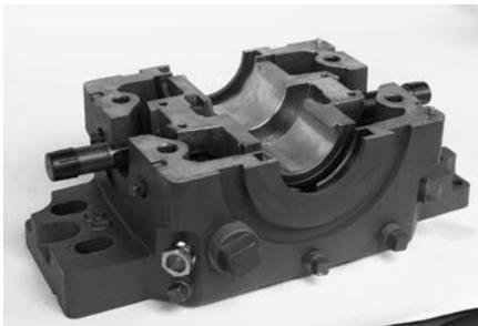
Because of the closely controlled liner to housing fit, it may be necessary to bolt the housing base down to allow the liner to slip into the housing seat. Do a preliminary alignment check at this time.
