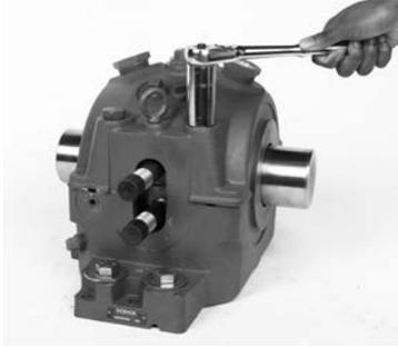
Insert the bolts, and torque to the values shown in Table 4.
