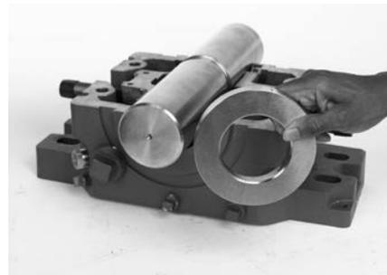
If clamp-on type thrust collar is used, make sure joints of collar are clean. Place both halves of thrust collar into shaft groove and tighten clamp screws alternately and evenly to torque value specified in Table 1.
