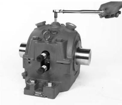
Next, tighten plunger screw to the mark. Remove shaft hold down and tighten plunger screw locknut.
