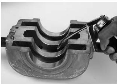
**WARNING:** If it ever becomes necessary to remove liner cap, make certain that both upper thrust plate halves remain in place next to the thrust collar. If a plate half should remain in the liner cap it can drop from the liner and cause injury.
