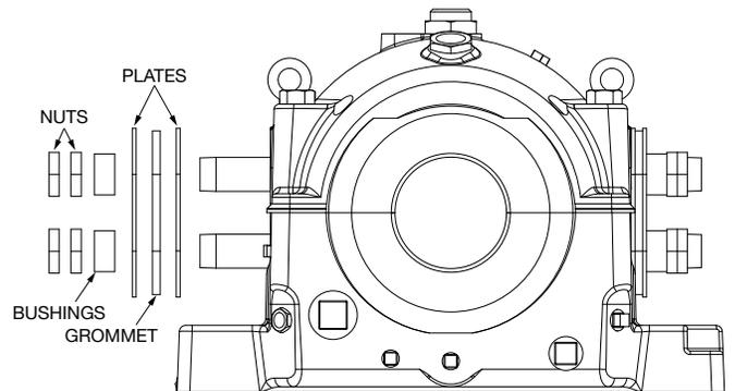
Install bushings and nuts on pipes (snug not tight).
