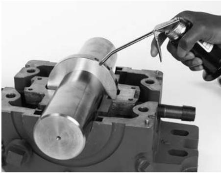
Place oil ring around outside of liner base and over shaft.
