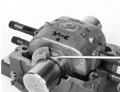
Install other half of seal and tighten screws to torque given in Table 3. Check to make sure the seal will slide along the shaft with minimum effort to allow for shaft expansion. Align the seal in the middle of the seal groove.
