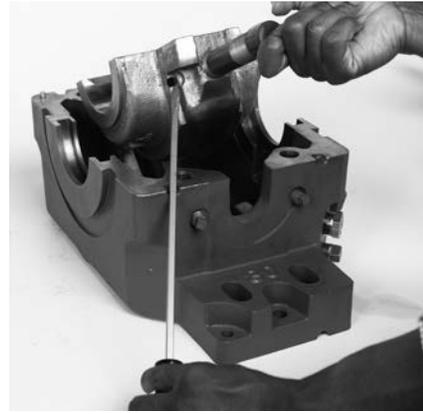
**Make sure the two thermocouple/RTD holes in the liner are aligned with the two thermocouple/RTD holes in the housing.** Apply oil to the liner bearing surface.
