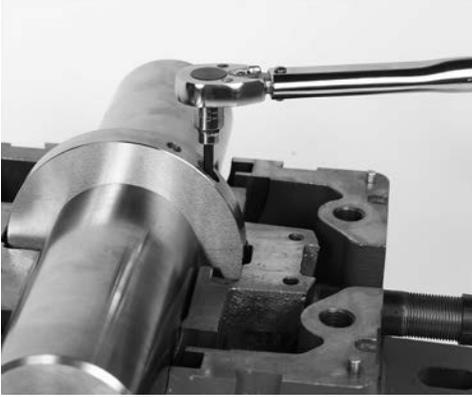
Oil shaft in the bearing area and CAREFULLY set shaft in place.
