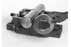
If clamp-on type thrust collar is used, make sure joints of collar are clean. Place both halves of thrust collar into shaft groove and tighten clamp screws alternately and evenly to torque value specified in Table 1.
