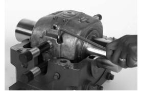
Install cap screws and tighten alternately to torque given in Table 2.
