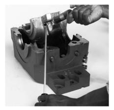
Make sure the two thermocouple/RTD holes in the liner are aligned with the two thermocouple/RTD holes in the housing. Apply oil to the liner bearing surface.
