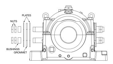
Install bushings and nuts on pipes (snug not tight).
