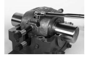
**NOTE:** If liner cap on non-expansion bearing will not drop into place, remove cap and reposition thrust plates tightly against thrust collar. Reinstall liner cap.
