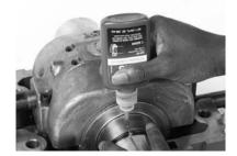
Apply a thin coat of heavy oil or light grease in the housing seal grooves to extend seal life.
