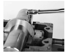
Oil shaft in the bearing area and CAREFULLY set shaft in place.
