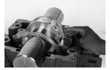
Install retainer washer in groove in liner base. Rotate plate until stopped by retainer washer.
