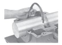
Install oil ring screws to insure they are secure. Repeat for second ring.
