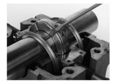
CAUTION: The bearing is not yet fastened in place and can be moved.
