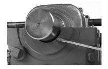
Tighten the four pedestal bolts to torque value given in Table 3. Shaft should rotate freely.
