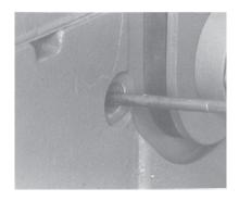
Check construction drawings to determine if coolant (water or air) is to be supplied to the bearings. Do not connect coolant pipes and bearing unless construction drawings and/or equipment instructions call for this. If no connection is required, pipes can be left open.
