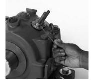
NOTE: ALL plumbing (oil and water) should be cleaned and flushed before being connected to the pillow block. These systems should be tested before the bearing is put into operation.
