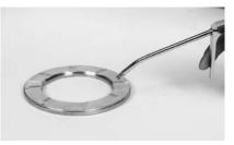
First, install the plate half without milled slots in the steel back. Press the babbitted face against the thrust collar and rotate plate around shaft into liner cavity.
