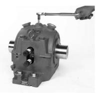
Next, tighten plunger screw to the mark. Remove shaft hold down and tighten plunger screw locknut.
