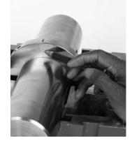
Tighten set screws to value specified in Table 1. Install and tighten jam screws 1/10 of torque specified for set screws.
