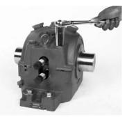
Insert the bolts, and torque to the values shown in Table 4.
