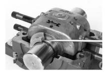
Apply RTV (not supplied) around each of the four housing bolt holes. This will prevent water from entering the bolt hole cavities.
