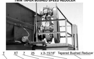
Torque-Arm Extra Case Normal Bore Bushina Gear Ratio Size Style Torque Size
