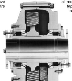
all reducer sizes from fractional to 700 HP. A tapered bore in both sides of the reducer's output hub snugs up against a matching taper on the outer surface of the bushing . . . Twin Tapered.
