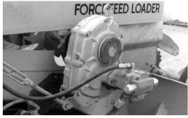
Tapered Bushed Reducer B 30 Vane Motor
