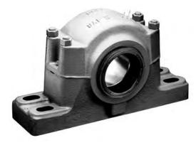
The SAF-XT pillow block has only one grease fitting. Bearings with costly, comparably effective auxiliary seals have up to three grease fittings. The single fitting speeds up lubrication, reduces chance for voids. Complete fill, bearing action, and configuration of reservoir assure maximum purging effectiveness. Grease relief channels result in self-centering positive contact seal. These factors make SAF-XT blocks easy to lubricate.
