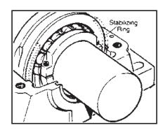
3. Place upper half of roller assembly in position and bolt on upper half of outer ring. Lower shaft and replace housing cap.
