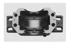
Large capacity oil sump lowers operating temperatures, undercut bearing seat allows full lateral travel of expansion bearing, prevents stabilizer ring from binding, makes installation easy.
