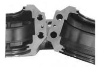
Offset dowels with matched numbers on cap and base joint simplify correct assembly.
