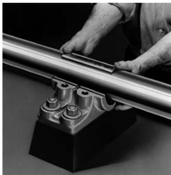
Lower half of new bushing is installed by relieving shaft pressure, prying out old bushing and rolling in new one.
