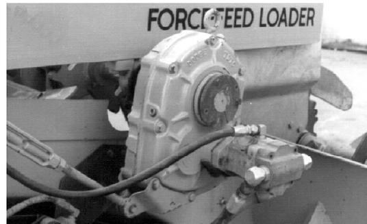
H XT 5 25 Tapered Bushed Reducer B 30 Vane Motor
