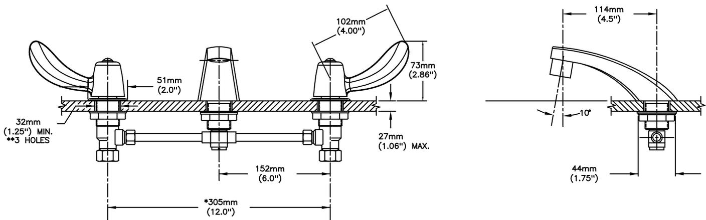
\* CAN BE CUT IN FIELD TO 152mm (6.0") MINIMUM
