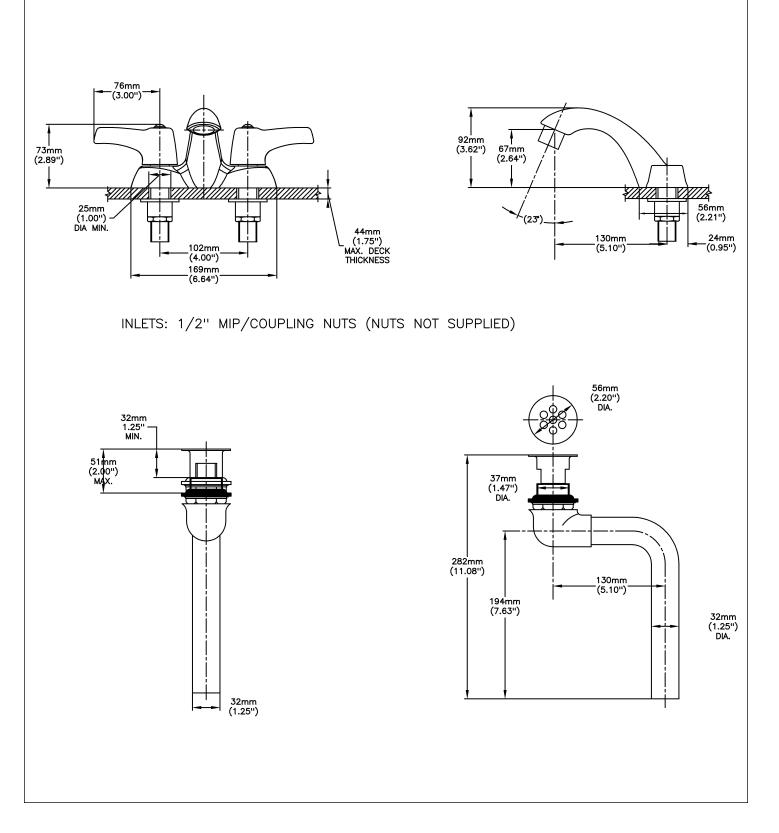
Delta reserves the right (1) to make changes to specifications and materials, and (2) to change or discontinue models, both without notice or obligation. Dimensions are for reference. Measurement may vary plus or minus 6mm(0.25"). Mounting locations are suggested only. Check with local codes for requirements in your area. This spec was produced May 31, 2017.
