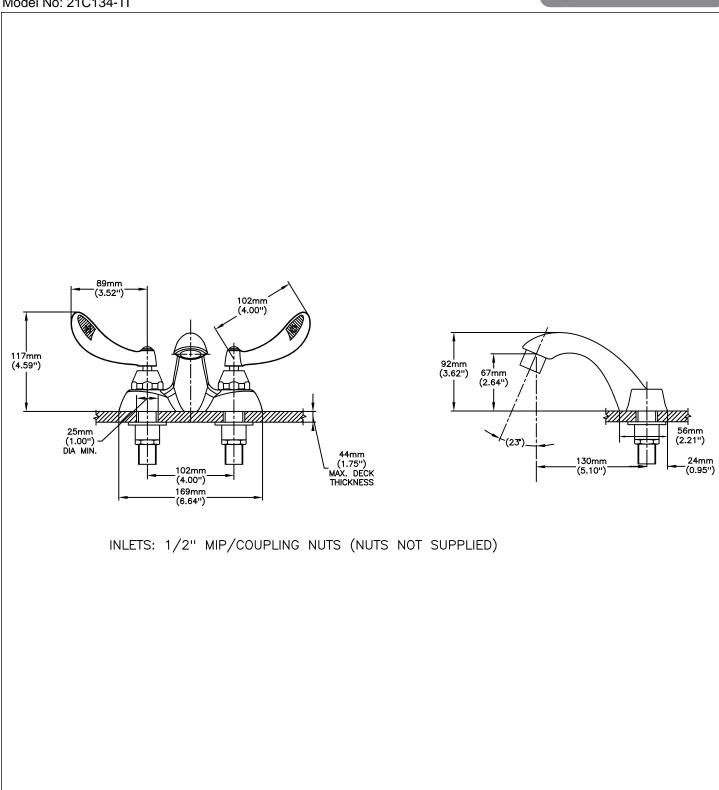
Delta reserves the right (1) to make changes to specifications and materials, and (2) to change or discontinue models, both without notice or obligation. Dimensions are for reference. Measurement may vary plus or minus 6mm(0.25"). Mounting locations are suggested only. Check with local codes for requirements in your area. This spec was produced May 25, 2017.
