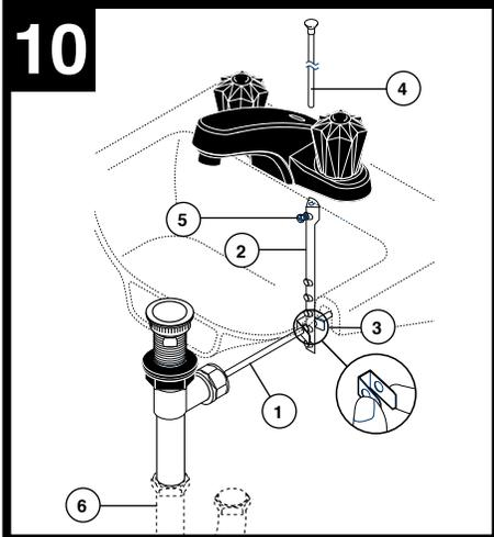
Attach horizontal rod (1) to strap (2) using clip (3). Install lift rod (4), tighten screw (5). Connect assembly to drain (6).
