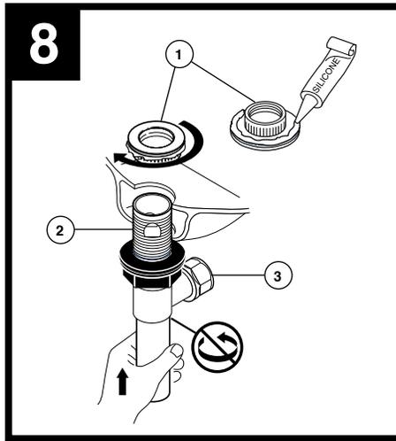
Apply silicone to underside of flange (1). Insert body (2) into sink. Screw flange onto body. Pivot hole (3) must face back of sink. Pull assembly down firmly and hold in place. DO NOT TWIST. Tighten nut, remove excess sealant.
