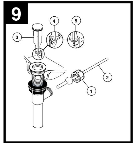
Remove pivot nut (1). Install horizontal rod (2) and stopper (3) as removable (4) or non-removable (5). Hand tighten nut (1).
