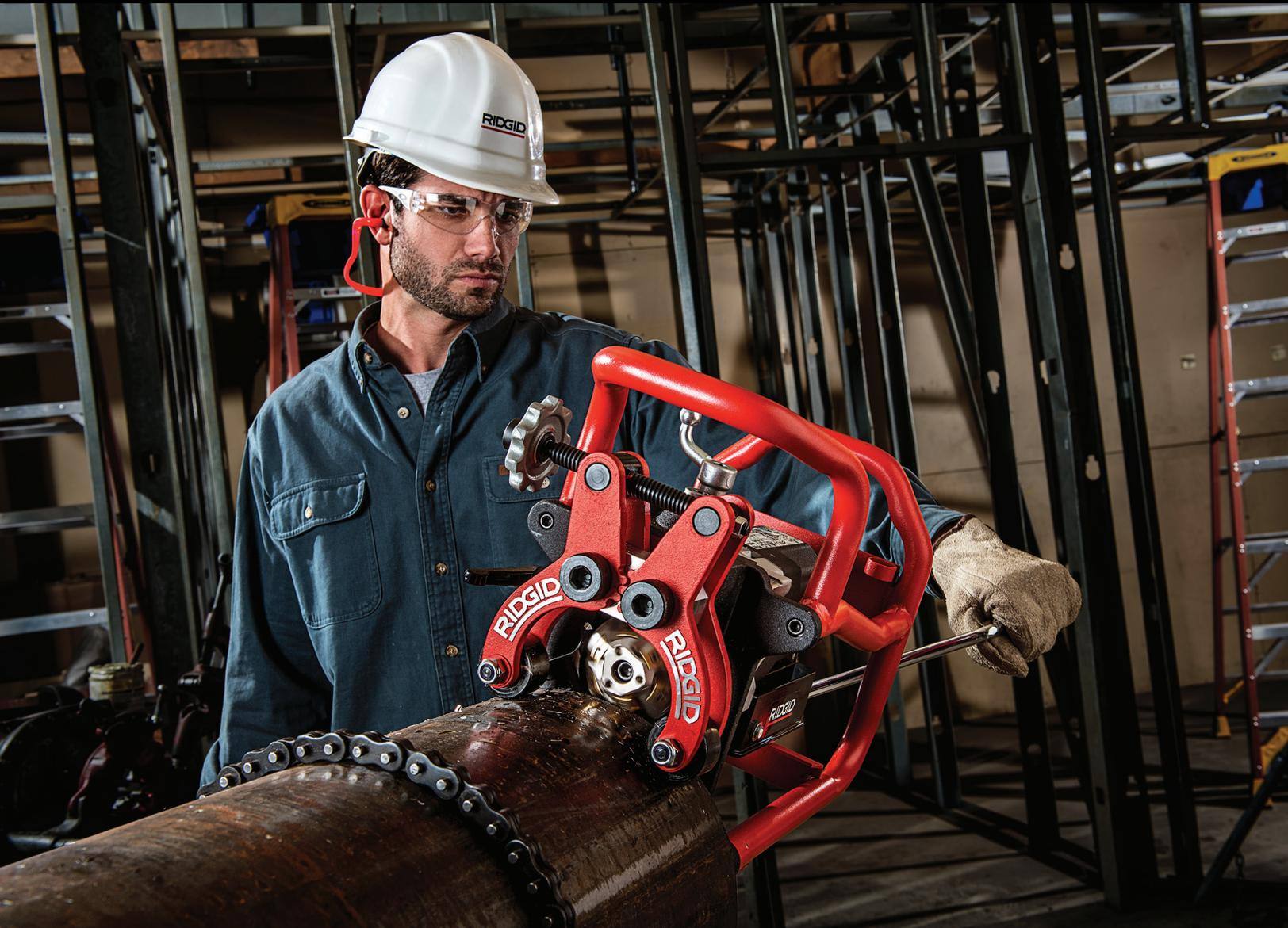
**Set-up and bevel 12" diameter schedule 40 pipe in one pass in under 2 minutes using the new B-500 Transportable Pipe Beveller. (Pipe capacity: 4" diameter and larger, 3/16" - 1/2" wall - See Specifications.)**
