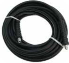
For use on either steam cleaner machines or combination steam cleaner/pressure washer machines. Handles hot water at 325°F (163°C) and 350 psi for Steam Cleaning Service, handles hot water at 250°F (121°C) and 3000 psi (2500 psi on 1/2") for Pressure Washer Service.
