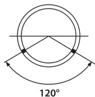
**Perforated PVC ASTM D 2729 Pipe**
