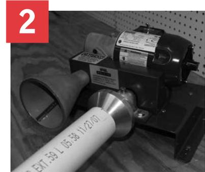
Chamfer (bevel) the end of the pipe  $10^{\circ}$  -  $15^{\circ}$ .
