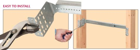
Bend bracket ends at 2-1/2" mark for use with 1/2" or 5/8" thick wall board. Ends can also be bent 90 degrees or backwards at 180 degrees as needed for inside.
