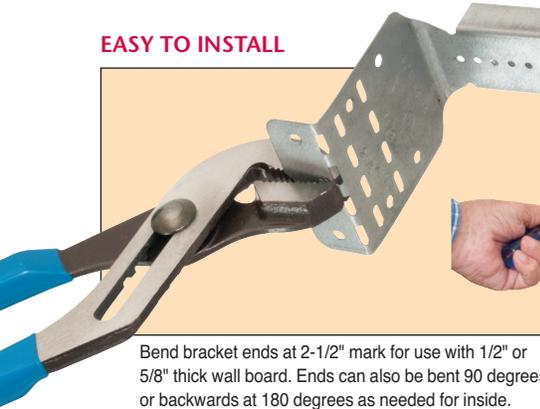
Bend bracket ends at 2-1/2" mark for use with 1/2" or 5/8" thick wall board. Ends can also be bent 90 degrees or backwards at 180 degrees as needed for inside mounting.
