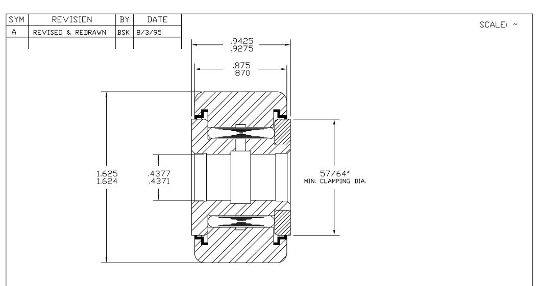
MAT'L: ST'D BEARING STEELS, SEALS - ACETAL. BEARING PACKED WITH GENERAL PURPOSE EP GREASE. RELUBE PROVISIONS WILL ACCEPT 3/16" DRIVE TYPE FITTINGS, PLUGS SUPPLIED FOR UNUSED HOLES. TOLERANCES
