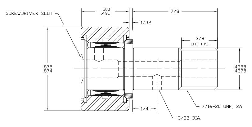
BASIC DYNAMIC CAPACITY - 1540 MAX. ALLOWABLE LOAD - 1600
