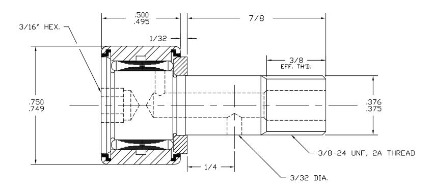
BASIC DYNAMIC CAPACITY - 1540 MAX. ALLOWABLE LOAD - 1360
