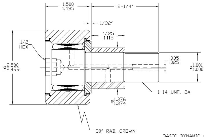
BASIC DYNAMIC CAPACITY - 15,280 MAX. ALLOWABLE LOAD - 16,650
