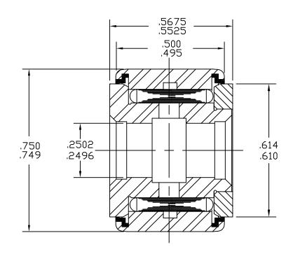
BASIC DYNAMIC CAPACITY - 1670 lbs. LIMITING SPEED - 3500 RPM
