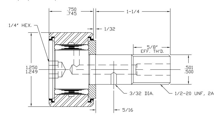
BASIC DYNAMIC LOAD RATING - 4470 MAX. STATIC CAPACITY - 4300
