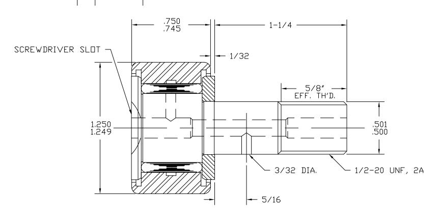
BASIC DYNAMIC CAPACITY - 3950 LBS. MAX. STATIC CAPACITY - 4250 LBS. REC. CLAMPING TORQUE - 350 IN-LBS.
