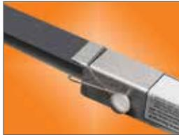
**Step 5:** With the line in the Start Slot, attach the spring to the belt. Note: For cog-belts the best place for the spring may be in a cog.
