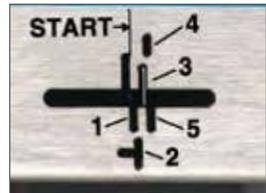
**Step 7:** Determine the required slot for your drive from Table 1. Tighten the belt until the line has moved to the designated slot. (In this picture the line is in Slot 3.)
