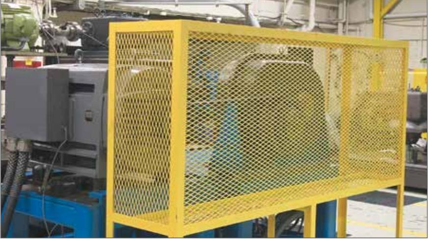
⚠️-6 **Foreign objects**, such as wood chips, can create havoc with v-belt drives. Belt breakage and turnover are the most common symptoms. Shielding the drive is a necessity. Belt guards with expanded metal screening are often used, but ventilation is sometimes sacrificed, possibly requiring additional cooling. Banded belts are sometimes effective, since they help keep debris from falling into the drive, however, if debris does get in, a banded belt can hold it in.
