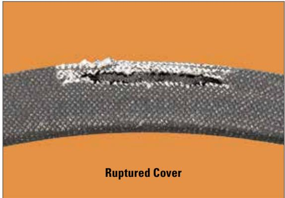
**⚠️-2 Belts rubbing against the metal guard or other obstruction** will be evidenced by cut or worn fabric on the back or upper edge of the v-belt. Often just replacing missing bolts in guard brackets will remedy this situation.
