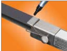
**Step 6:** Scribe a line at the spring end of the Tension-Finder. Use this line as a reference point in case the spring slips off the belt.
