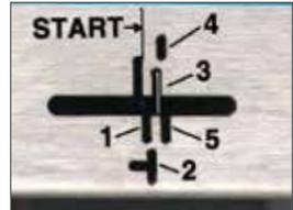
**Step 7:** Determine the required slot for your drive from Table 1. Tighten the belt until the line has moved to the designated slot. (In this picture the line is in Slot 3.)
