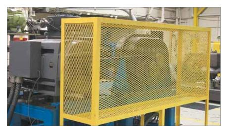
▲ 6 Foreign objects, such as wood chips, can create havoc with v-belt drives. Belt breakage and turnover are the most common symptoms. Shielding the drive is a necessity. Belt guards with expanded metal screening are often used, but ventilation is sometimes sacrificed, possibly requiring additional cooling. Banded belts are sometimes effective, since they help keep debris from falling into the drive, however, if debris does get in, a banded belt can hold it in.
