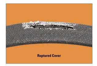
▲-2 **Belts rubbing against the metal guard or other obstruction** will be evidenced by cut or worn fabric on the back or upper edge of the v-belt. Often just replacing missing bolts in guard brackets will remedy this situation.
