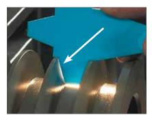
Worn Groove Sidewalls
