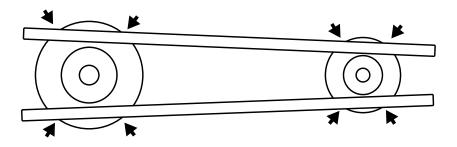
Parallel (offset) – shafts are parallel; sheaves not in line
