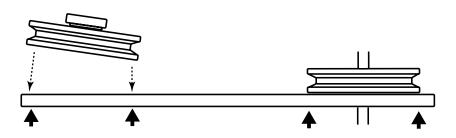
Vertical Angular – shafts in same vertical plane but not parallel To Check: Use laser alignment tool or place straightedge midway between the hub and the outside diameter of both sheaves. Repeat on opposite side of second shaft. The straightedge should touch at all four points shown below. To Correct: Use shims under motor base in front or rear of motor, depending on type of correction required.
