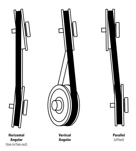
Horizontal Angular (toe-in/toe-out) – shafts in same horizontal plane but not parallel To Check: Use laser alignment tool or straightedge near sheave centers. To Correct: Loosen motor mounting bolts and rotate motor until all four points touch straightedge.
