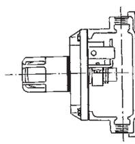
Add Suffix as listed below. Transformer clamps directly to pilot light barrel. Only one pilot light transformer assembly per one gang body.
