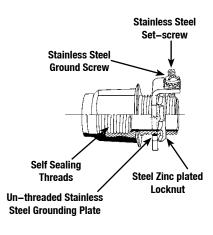
Optional union hubs are of stainless steel and Noryl<sup>®</sup> Construction. Ground plate is stainless steel and not threaded. Hub spins freely for ease of installation; then steel locknut is tightened to secure hub.
