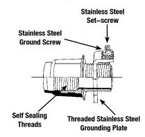
Standard hubs are of stainless steel and Noryl<sup>®</sup> construction. Stainless steel ground plate is threaded and includes stainless steel set-screw and ground screw.
