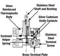
The standard Labyrinth switch is available with universal contacts (1 NO/1 NC). The switch is a UL recognized component and is rated for A600 heavy pilot duty (AC) and P150 (DC) as defined by UL 508. Hazardous Location ratings include Class I, Division 2, Groups B, C, D.
