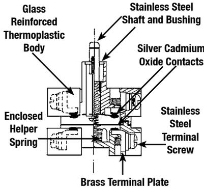
The standard Labyrinth switch is available with universal contacts (1 NO/1 NC). The switch is a UL recognized component and is rated for A600 heavy pilot duty (AC) and P150 (DC) as defined by UL 508. Hazardous Location ratings include Class I, Division 2, Groups B, C, D.
