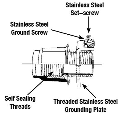
Standard hubs are of stainless steel and Noryl® construction. Stainless steel ground plate is threaded and includes stainless steel set-screw and ground screw.
