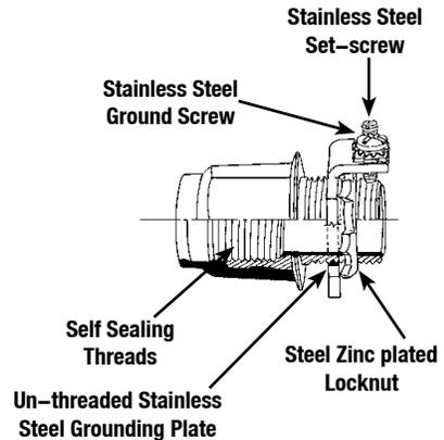
Optional union hubs are of stainless steel and Noryl® construction. Ground plate is stainless steel and not threaded. Hub spins freely for ease of installation; then steel locknut is tightened to secure hub.
